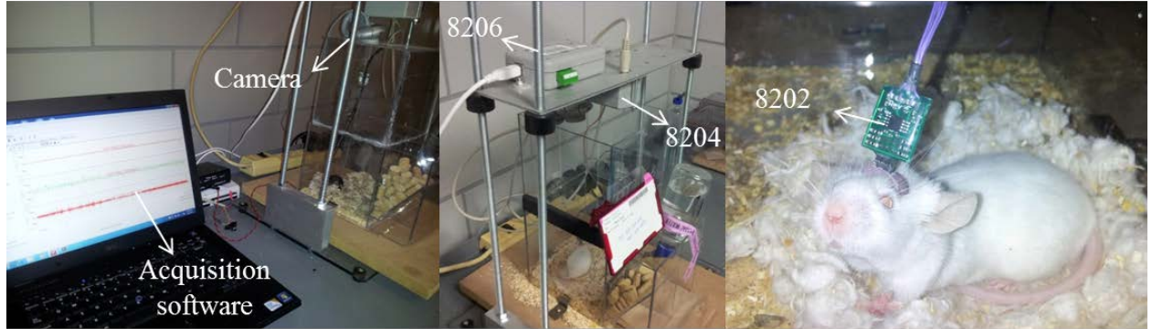
Figure 2.3 Data acquisition system. The preamplifier (#8202) is attached to the animal's headmount and provide initial 50x amplification. A commutator (#8204) connects the preamp to the data acquisition system (#8206). After a final amplification and conditioning by 8206, digital data are recorded using Sirenia™.
